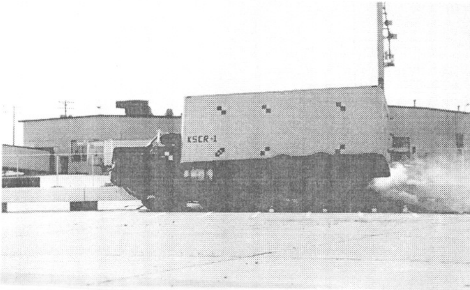
Figure 19. Full-Scale Vehicle Crash Test, KSCR-1
