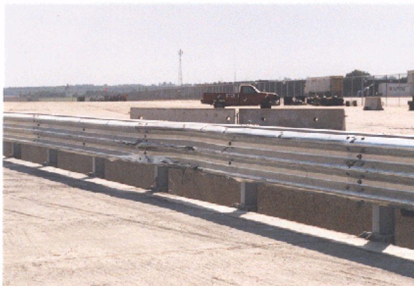
Figure 6. Impact Location, Vehicle Damage, and Bridge Railing Damage, Test STCR-1.
