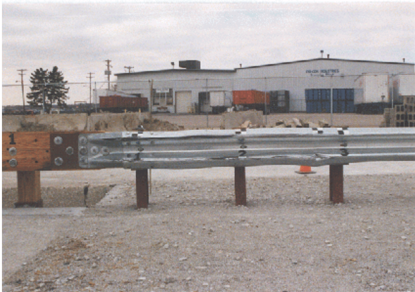
Figure 11. Impact Location, Vehicle Damage, and Approach Guardrail Transition Damage, Test WRBP-2.
