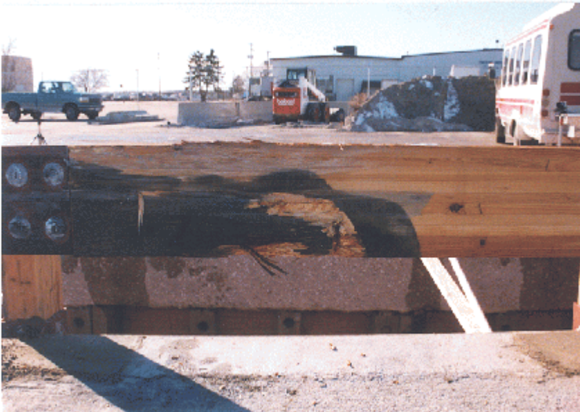
Figure 10. Impact Location, Vehicle Damage, and Bridge Railing Damage, Test WRBP-1.
