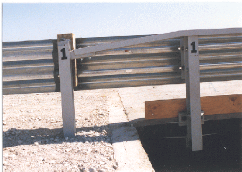
Figure 1. Steel Thrie Beam with Channel Bridge Railing and Thrie Beam with Channel Transition, System No. 1.
