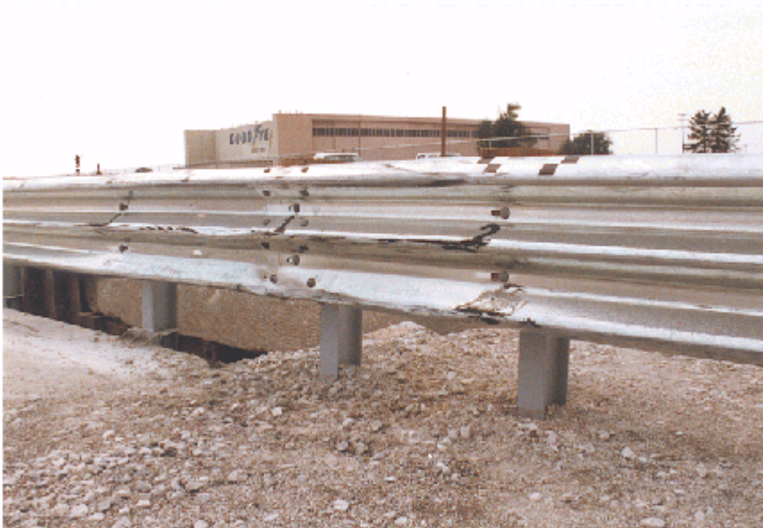
Figure 7. Impact Location, Vehicle Damage, and Bridge Railing Damage, Test STCR-2.
