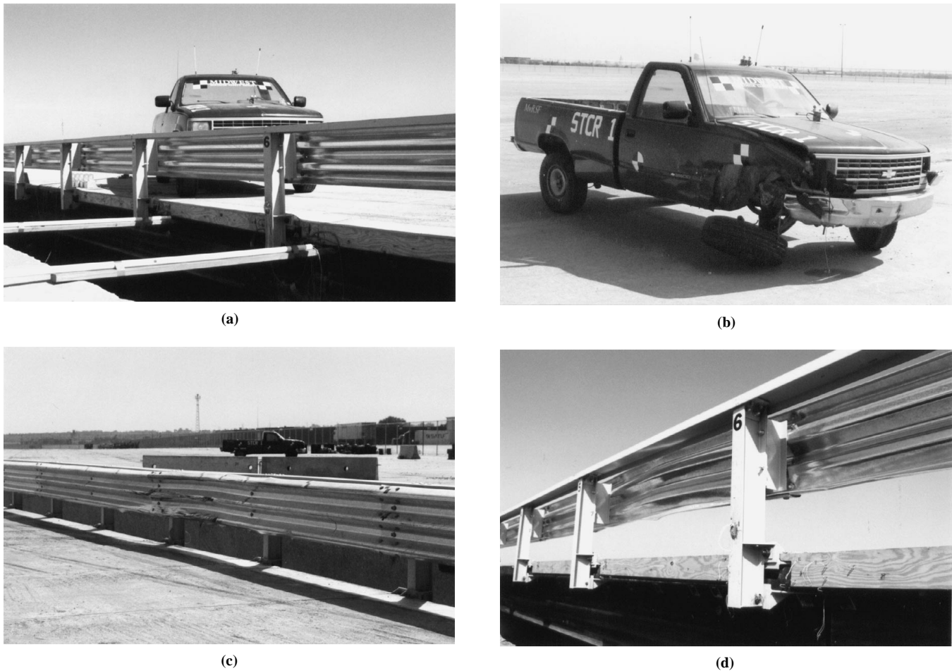
FIGURE 6 Test STCR-1: (a) impact location, (b) vehicle damage, and (c, d) bridge railing damage.
