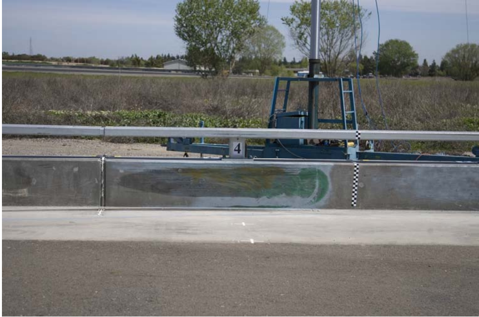
Figure 2-28 – Type 90 bridge rail face after Test 633
