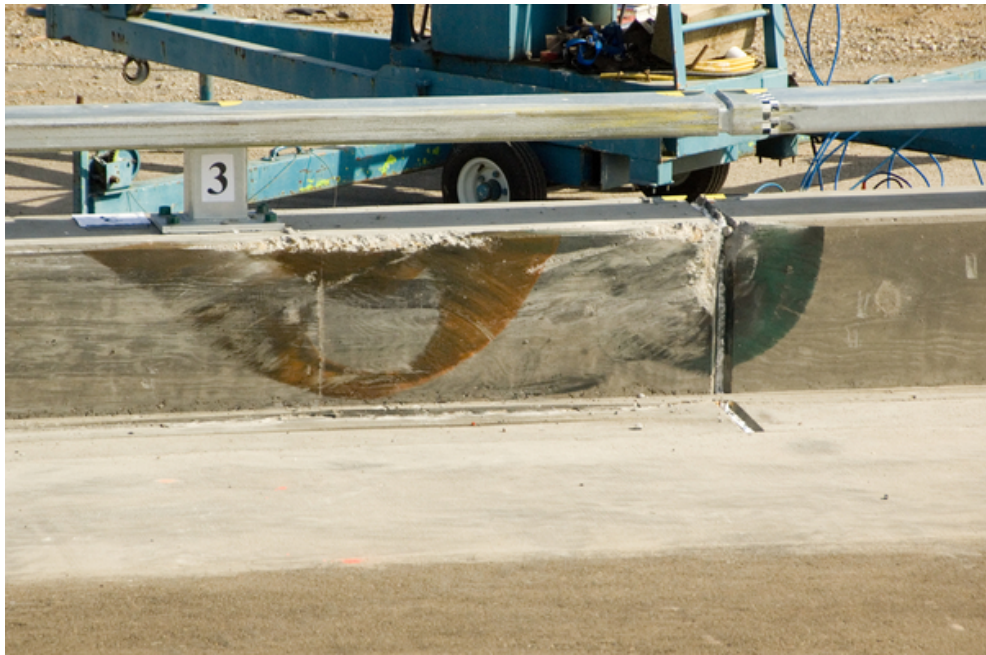
Figure 2-13 – Type 90 barrier face after Test 631
