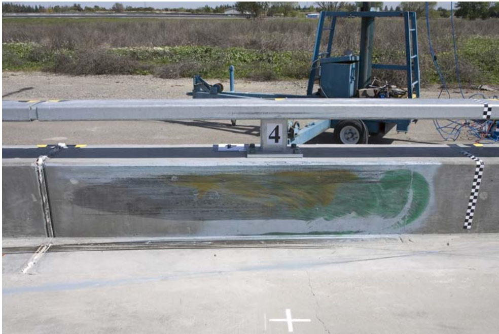
Figure 2-29 – Barrier face scraping after Test 633
