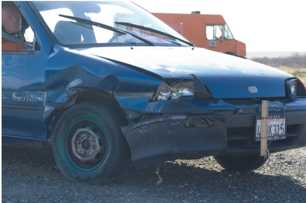
Figure 2-18 – Front right corner of test vehicle after Test 632
