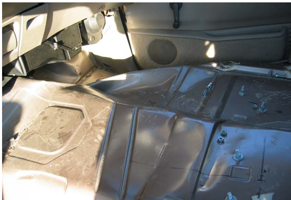
Figure 2-9 – Floorboard deformation of test vehicle after Test 631
