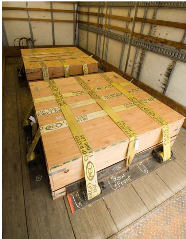
Figure 2-38 – Ballast strapped down in cargo bed of test vehicle after Test 634
