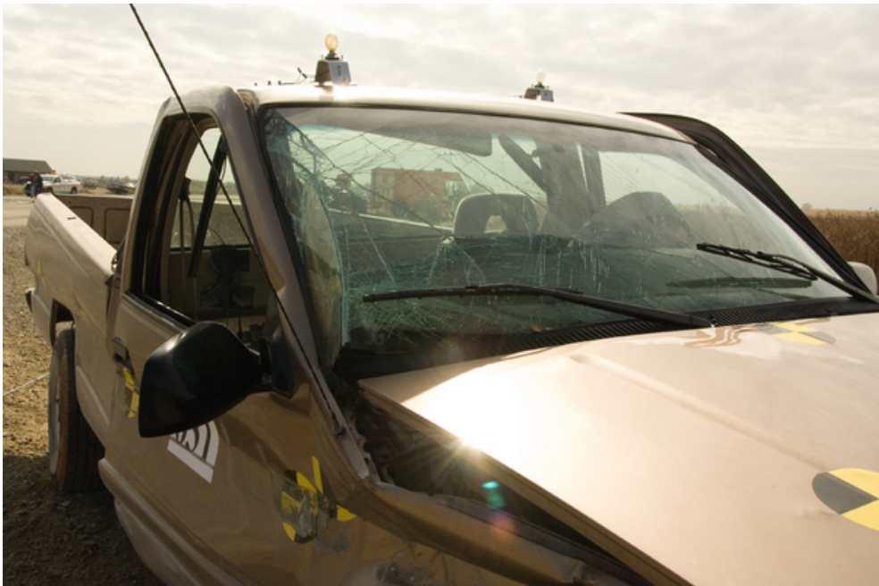
Figure 2-11 – Vehicle windshield after Test 631
