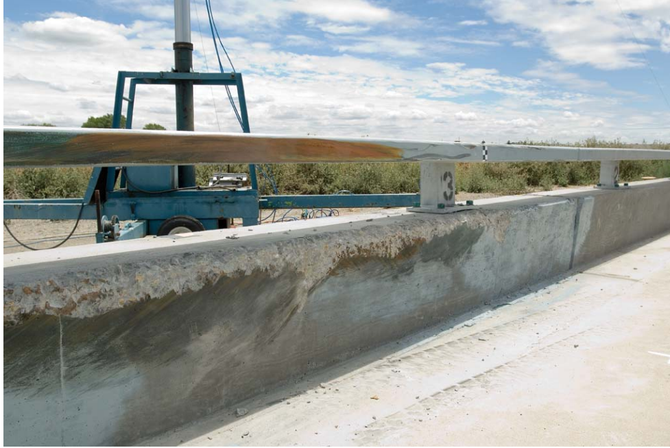
Figure 2-37 – Type 90 barrier face after Test 634
