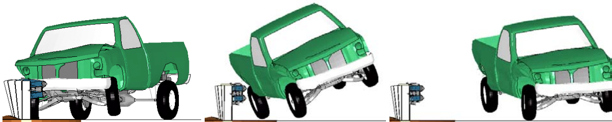
Figure 21: Sequential views of the simulated Test 3-11 impact event on the modified GR-2.2 with two-tube backup (posts in soil)
