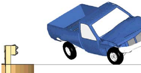
Figure 50: Sequential views of the NCHRP Report 350 Test 3-11 analysis of the modified GR-2.2 with nested w-beam rails and standard GR-3.4 transition for impact.
