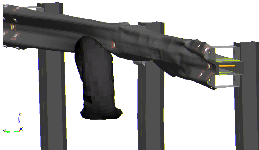
Figure 13: View from the F.E. analysis illustrating the interaction of the tire with the guardrail
