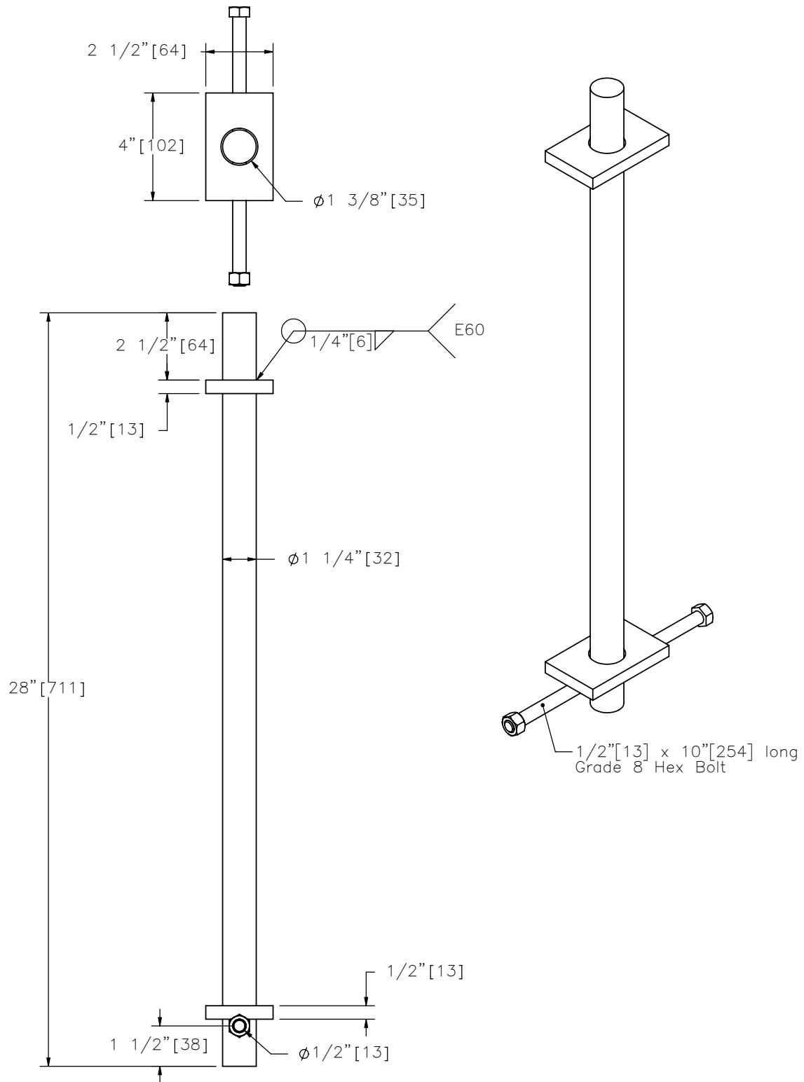
TEMPORARY BARRIER CONNECTOR PIN WITH RETAINING BOLT
